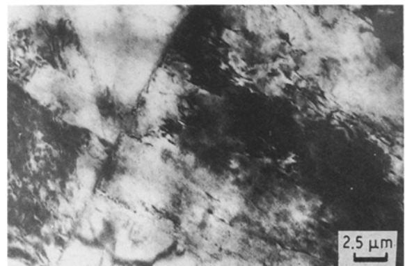
Figure 6 Transmission electron micrograph showing development of sub-boundaries after isothermal holding at 1173 K for 60 min.
